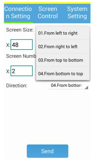
① Screen size: Setting the size of the smallest splicing unit of the entire screen, X represents a unit of width, and Y represents a unit of height.
